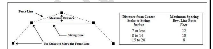
Determine line post spacing on curves based on the sharpness of the curve.
